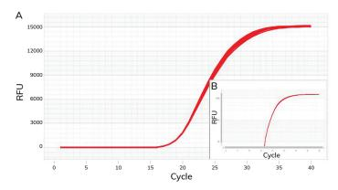
Unparalleled uniformity. Amplification curves for 96 replicates shown on a linear plot (A) and a logarithmic plot (Figure B). In each well,  $10^5$  copies of GAPDH template were amplified. Average Cq = 19.1, Coefficient of variance (Cv)= 0.002.
